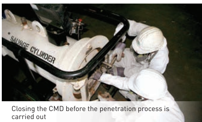
Tightening the entry point of flammable gas into Incineration Plant
