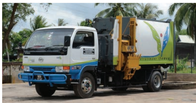
MPAR equipped with side loader robotic arm and CCTV
